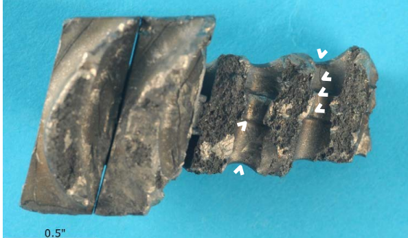
Figure 6. Views showing the airfoil and identify cracks in the rivet holes. (Honeywell)
