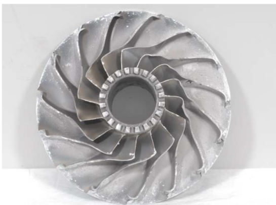
Fig. 3 – Damage of 2 nd Stage Impeller.
