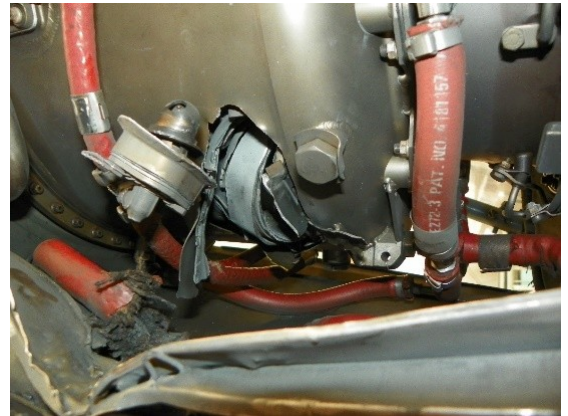
Fig. 1 - Engine No. 2 and the detail of the combustor plenum penetration.
