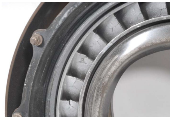
Fig. 4 – 1st Stage Nozzle - Cracks on Trailing Edges
