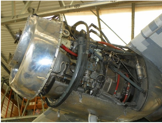
Fig. 1 - Engine No. 2 and the detail of the combustor plenum penetration.
