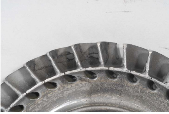
Fig. 6 – 1 st Stage Turbine Wheel – Leading Edge.
