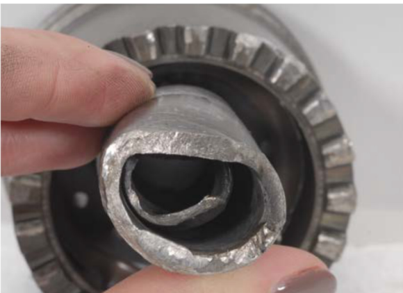
Fig. 8 – Fractured Main Shaft and Torsion Shaft
