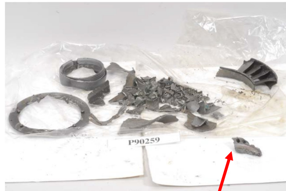
Fig. 3 Hole in Combustor Plenum Housing at 7:00 O'clock and debris - Fragment of a Turbine Rotor (source Honeywell).
