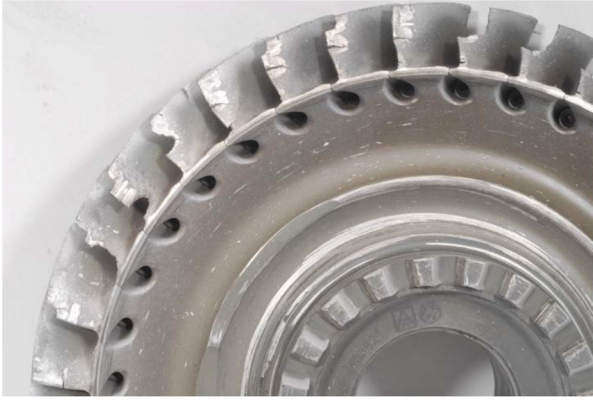
Fig. 5 – 1 st Stage Turbine Wheel - Aft View.
