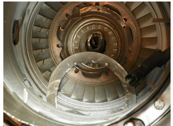
Fig. 2 - Rear view of engine No. 2 and detail of damage.
