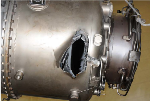
Fig. 3 Hole in Combustor Plenum Housing at 7:00 O'clock and debris - Fragment of a Turbine Rotor (source Honeywell).
