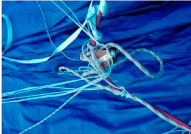
Fig. 7 – Entangled control cables and lines.
