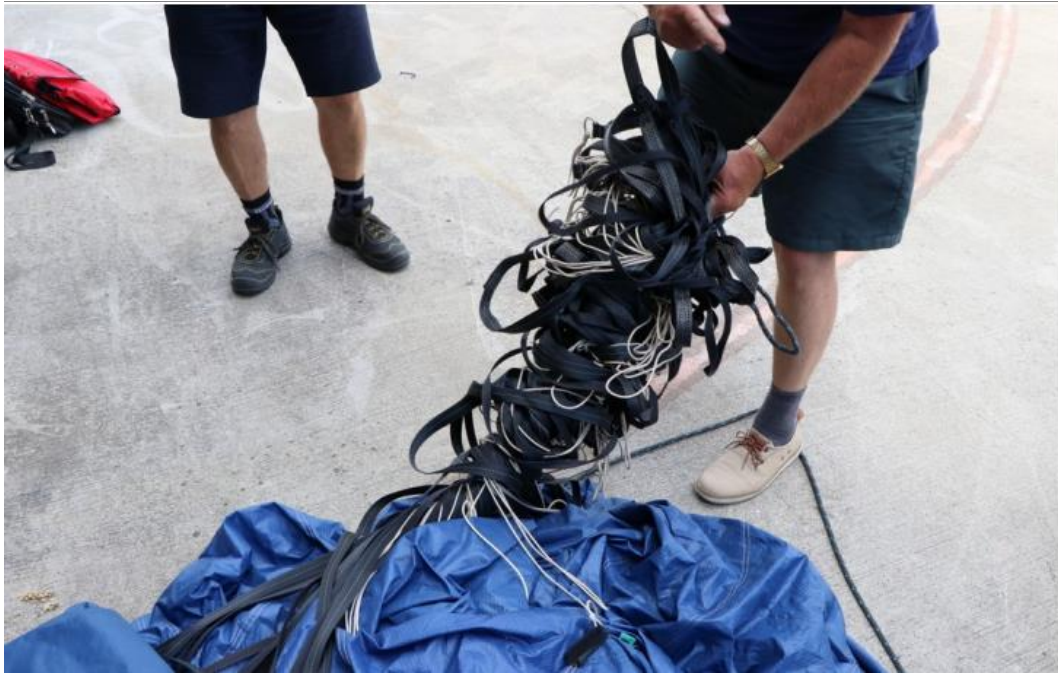
Fig. 5 – The control lines, straps, and centring lines condition during the inspection of the hot-air balloon
