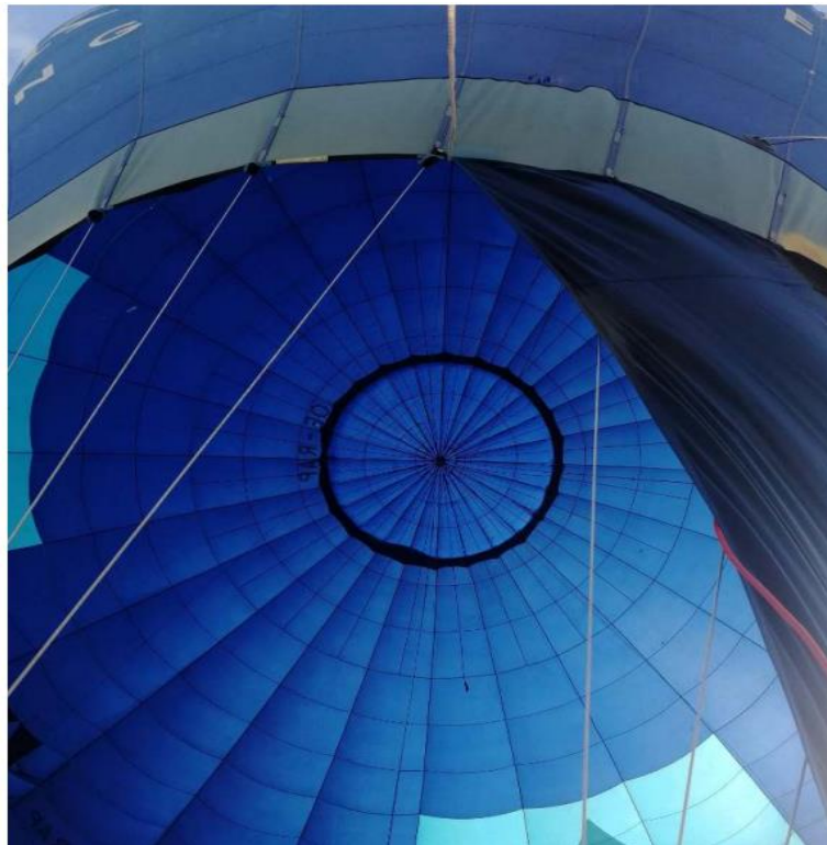
Fig. 9 – View of the deflation mechanism assembly inside the envelope
