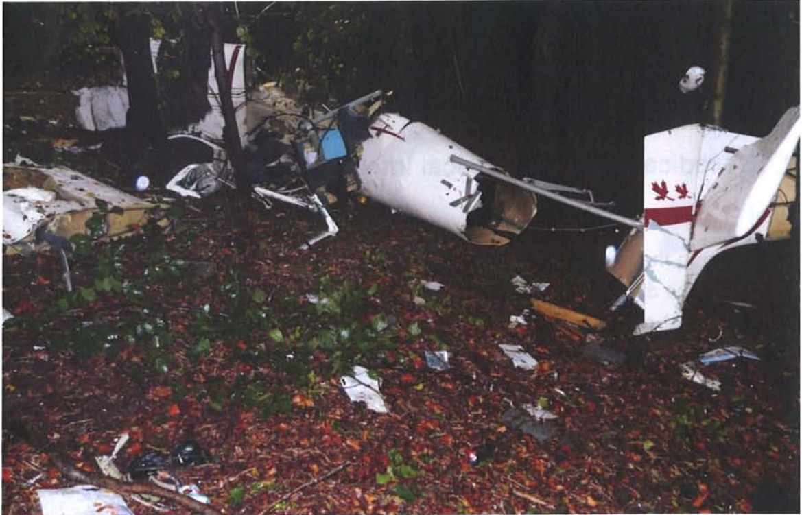
High degree of destruction due to the collision with trees
