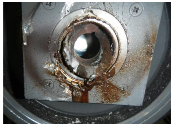
Fig. 3 Broken fan shaft cone of the R22 helicopter
