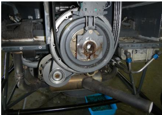
Fig. 3 Broken fan shaft cone of the R22 helicopter
