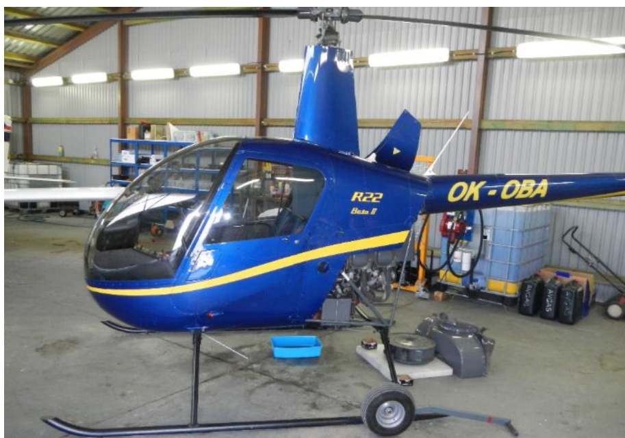
Fig. 1 Helicopter after the incident with the engine cooling fan removed
