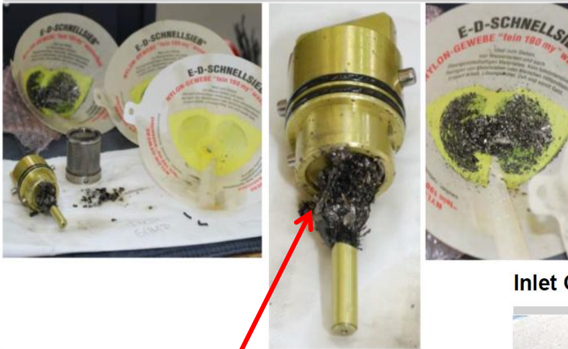
Metallic chips on the forward sump magnetic chip detector and strainer.
