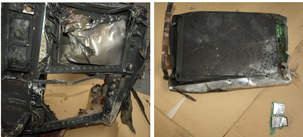
Fig. 12 – Both the MFDs destroyed by fire (left) and the MFD with the double data card slots (right)
