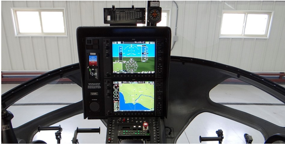
Fig. 3 – Garmin G 1000H system integrated into the instrument panel
