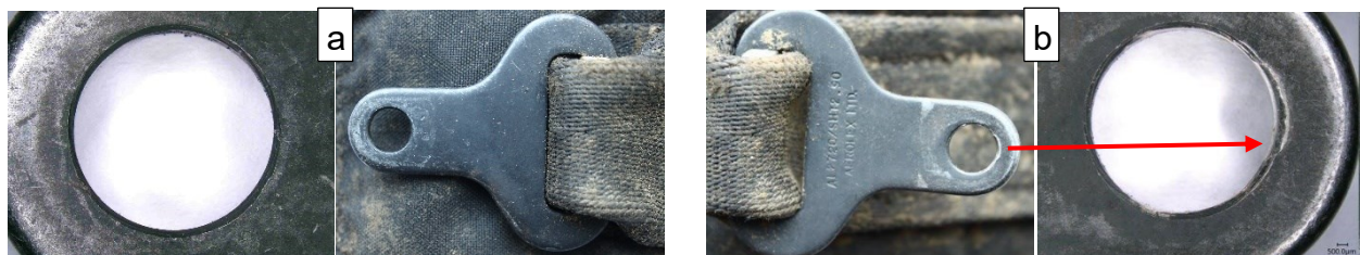
Fig. 5 – The right clamp on the lap seat belt; (a) front part of the right clamp; (b) rear part of the right clamp.
