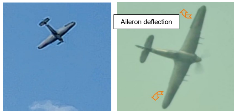
Fig. 2 – Aileron deflection against the rolling movement in a descending turn.
