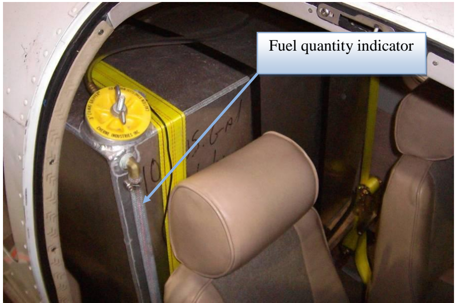
Fig 6. Auxiliary tank and fuel quantity indicator position
