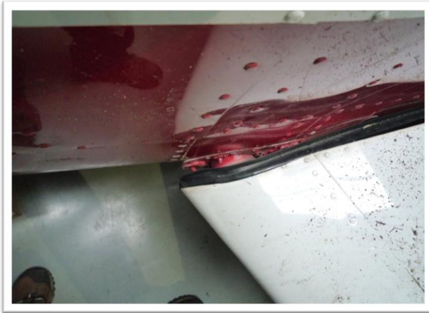
Fig. 7 Damaged of the left wing/fuselage midsection attachment
