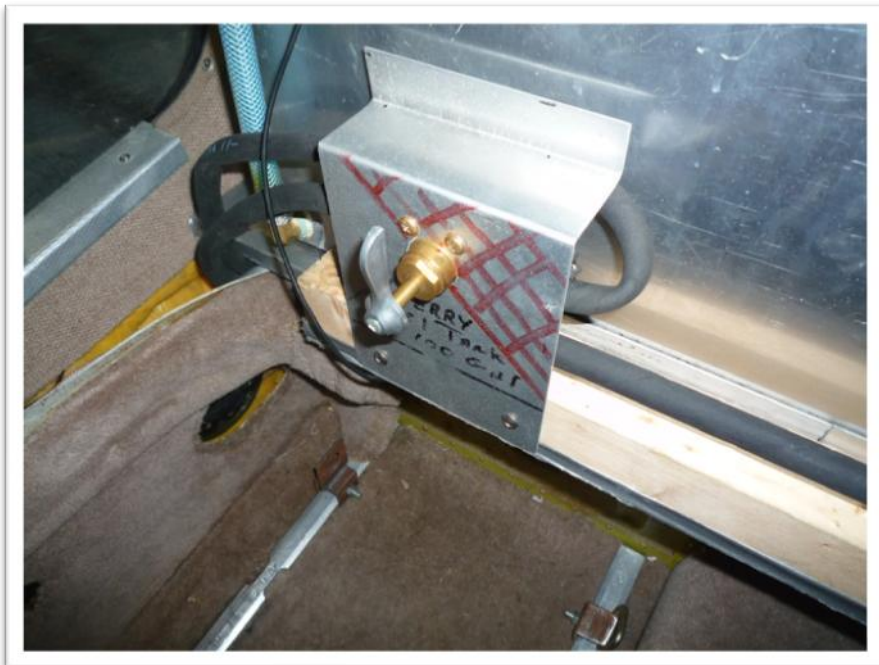
Fig. 10 Position of the lever auxiliary fuel cock after forced landing
