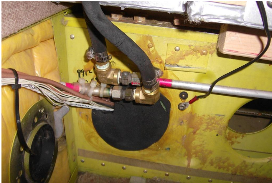
Fig 7. Auxiliary fuel system instalation place
