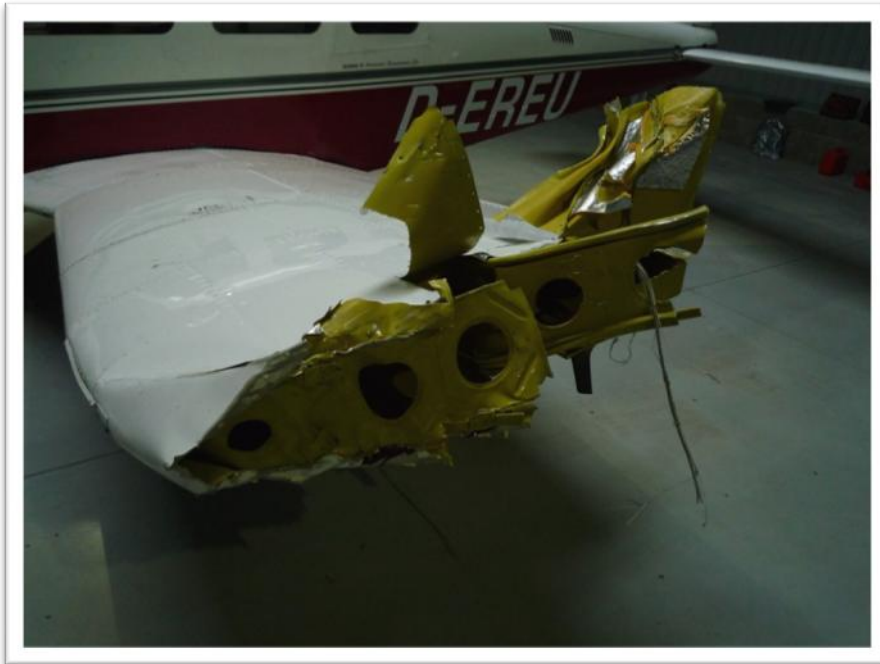
Fig. 3 Damaged of left wing
