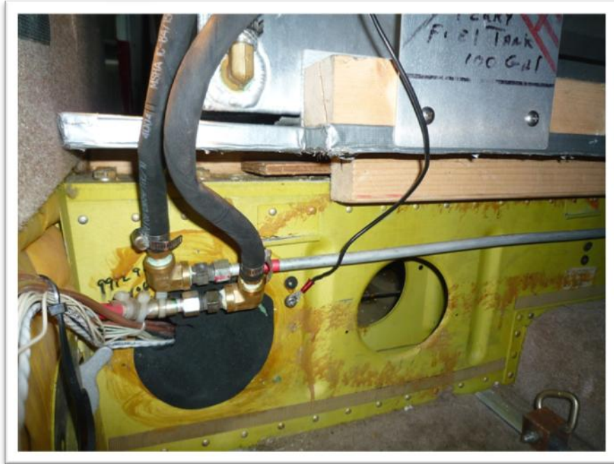
Fig. 9 Auxiliary fuel system instalation place
