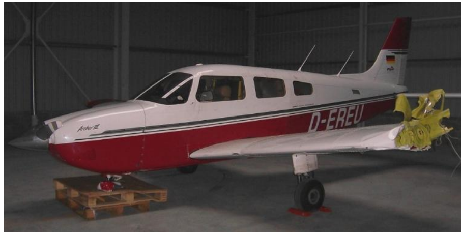
Fig. 4 Damage of the airplane PA-28-181 D-EREU
