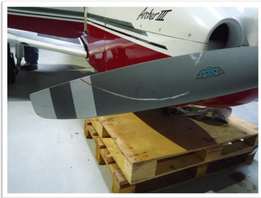
Fig. 5 Damaged of ride side the aircraft propeller
