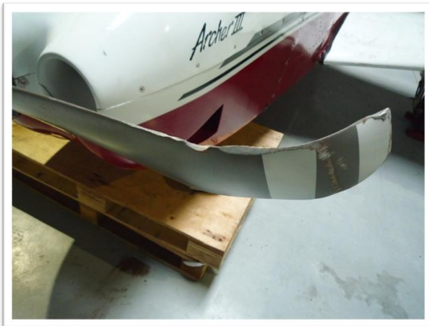
Fig. 6 Damaged of left side the aircraft propeller
