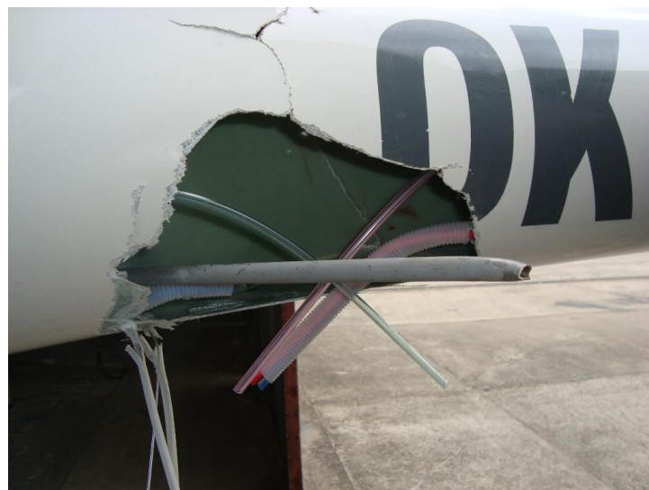
Damaged of left side fuselage
