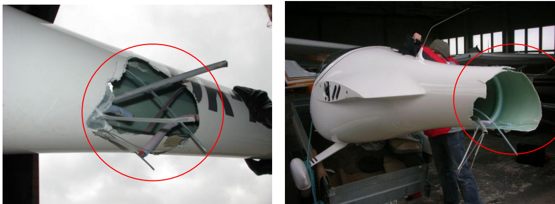
Damaged of fusselsage
