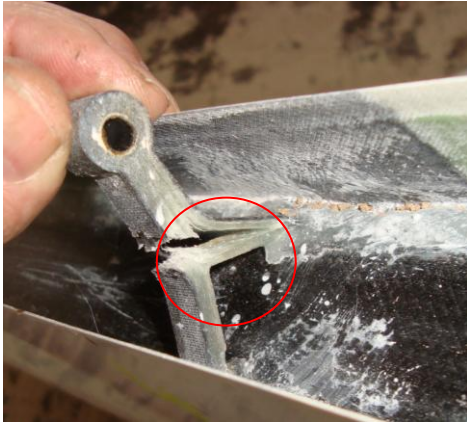
Damage of hinge and elevator control lever
