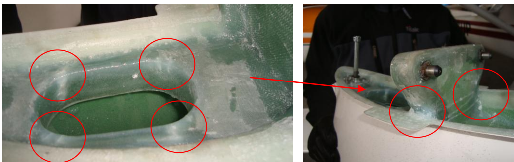
Damage of connection between the elevator bracket and the fin
