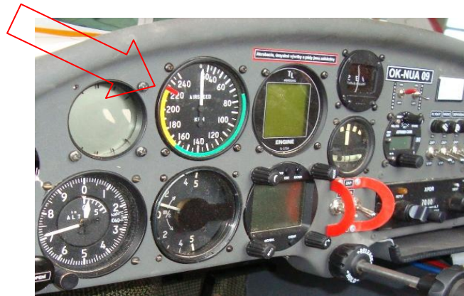
Colour-codet of max. speed on microlight airspeed indicator Reg.mark OK-NUA 09
