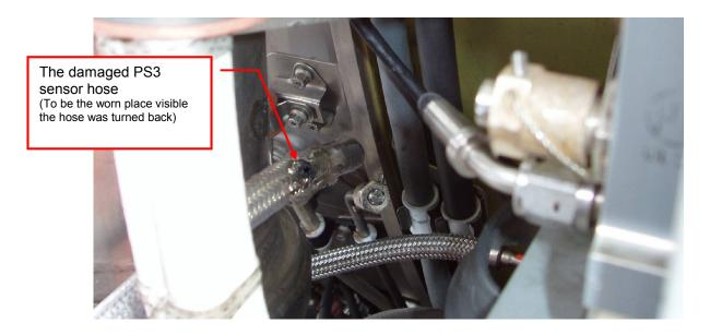
The PS3 sensor hose had been replaced and the subsequent engine test run showed the engine was working free and clear.
