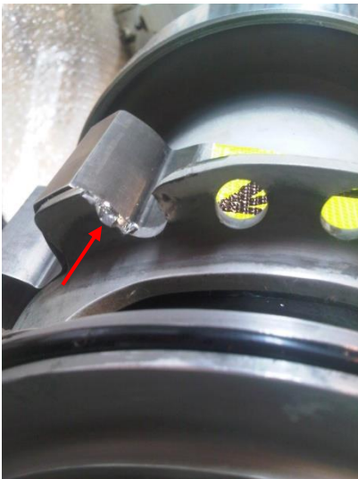
Pic. 3,4 Damage to the steering mechanism - p/n 200429305
