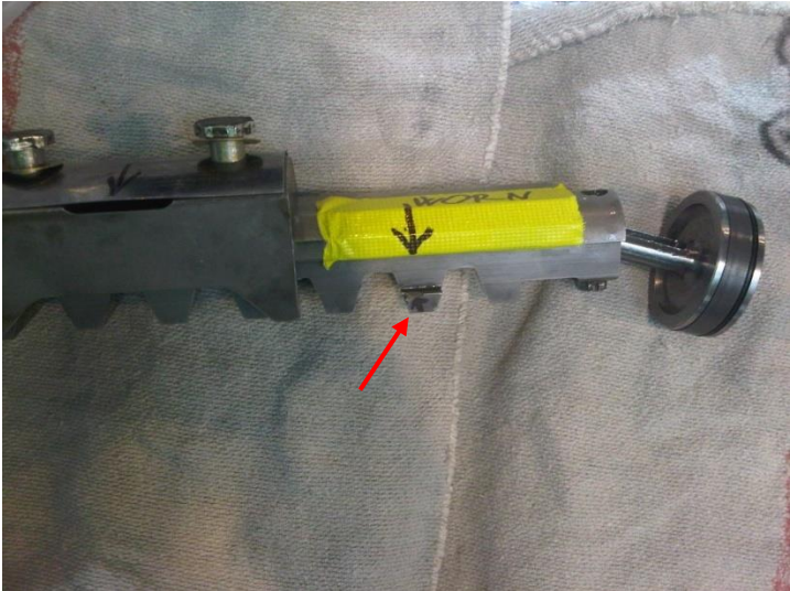
Pic. 3,4 Damage to the steering mechanism - p/n 200429305
