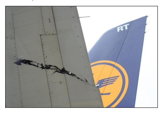
Fig. 3 Damage to A321-131 left rudder and stabiliser.
