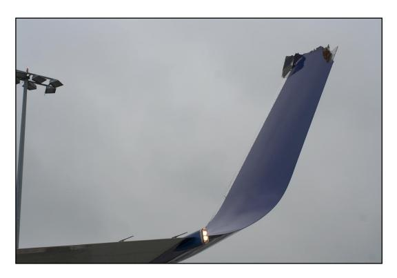
Fig. 5 Damage to B737-8BK right wing winglet.
