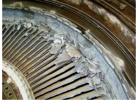
the 2 nd to 4 th LPT stages blades were damaged too
