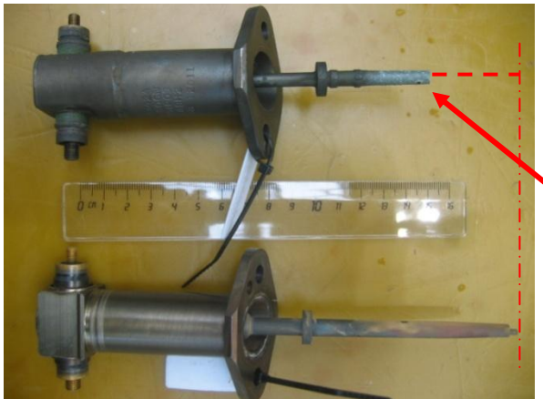
measuring probe EGT, 1/3 of the probe body was missing
