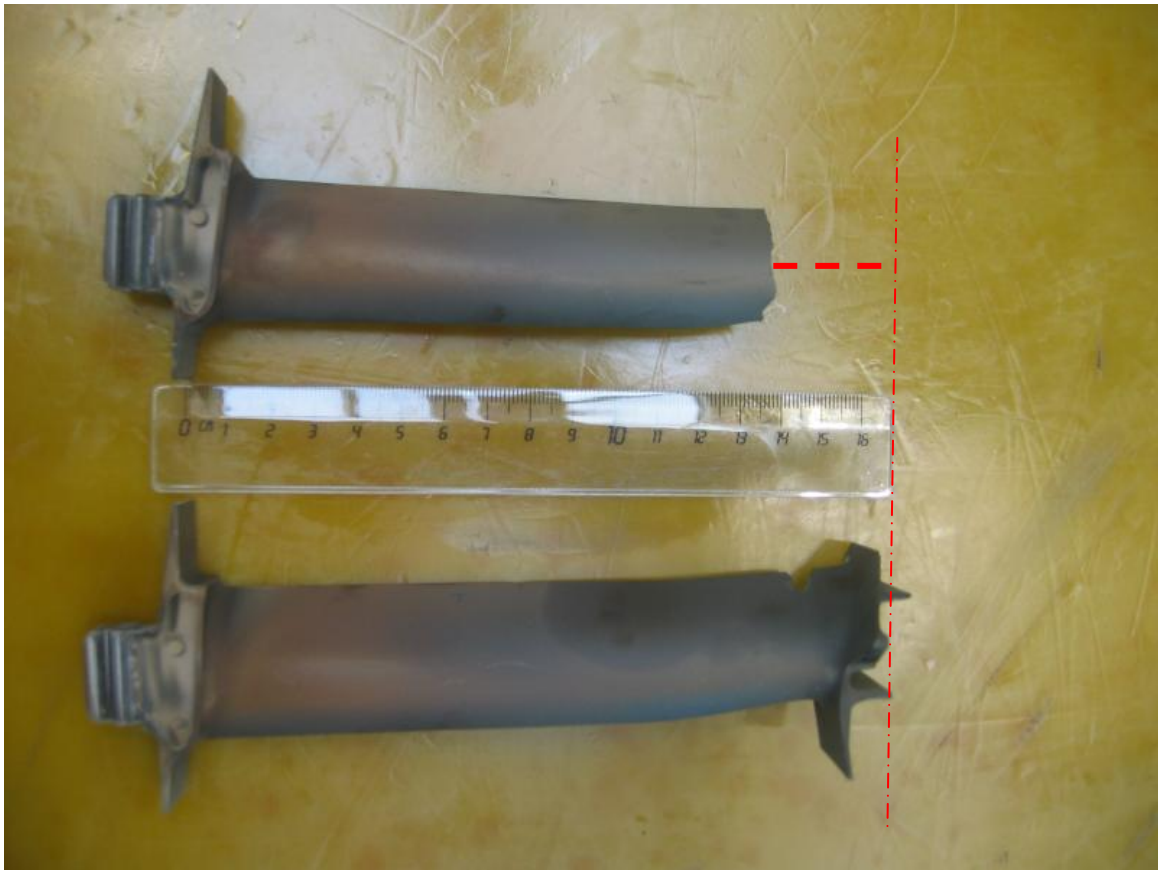
1/5 of the working part of a blade of LPT's first stage was broken off
