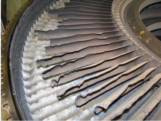
the 2 nd to 4 th LPT stages blades were damaged too
