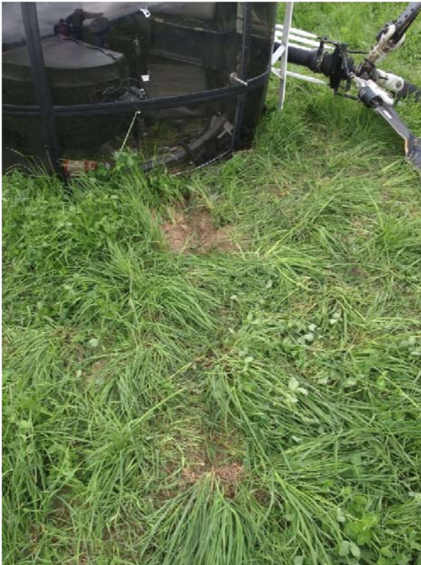
The evidence of impact of main rotor blades
