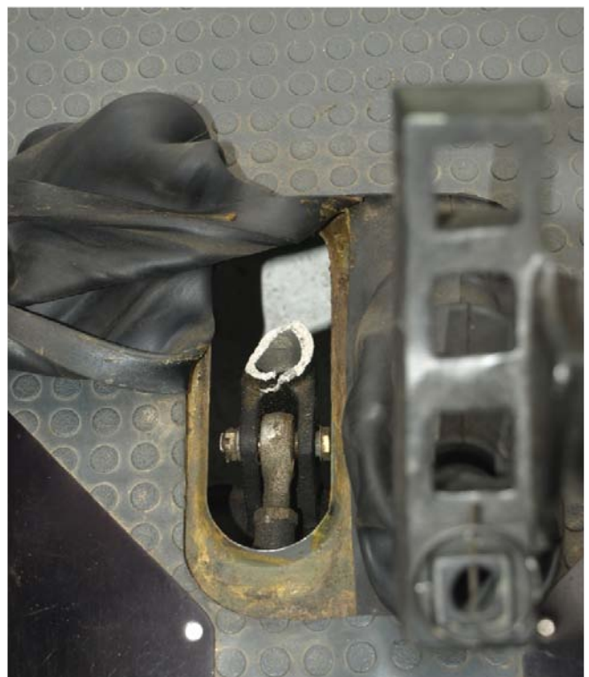
The broken socket of the left pedal
