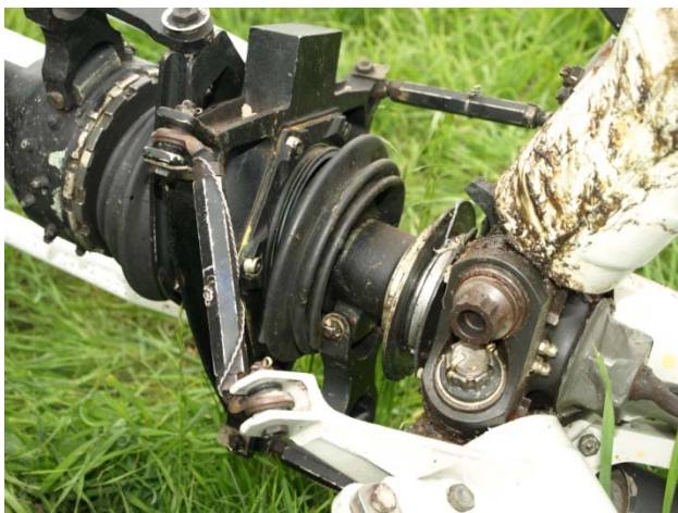
Damaged blade control rods
