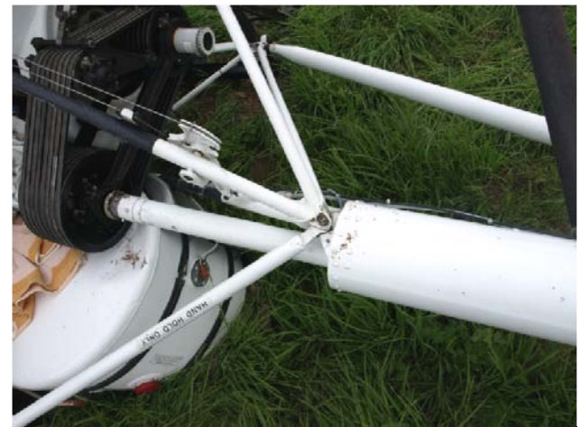
The transmission shaft and boom
