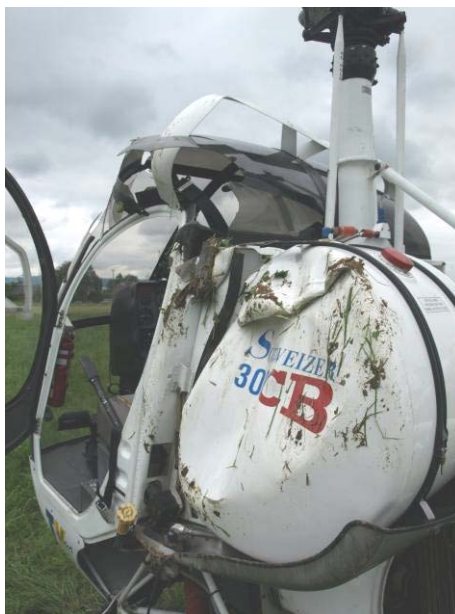
Fig. 2 Damaged left side of the helicopter OK-XIS
