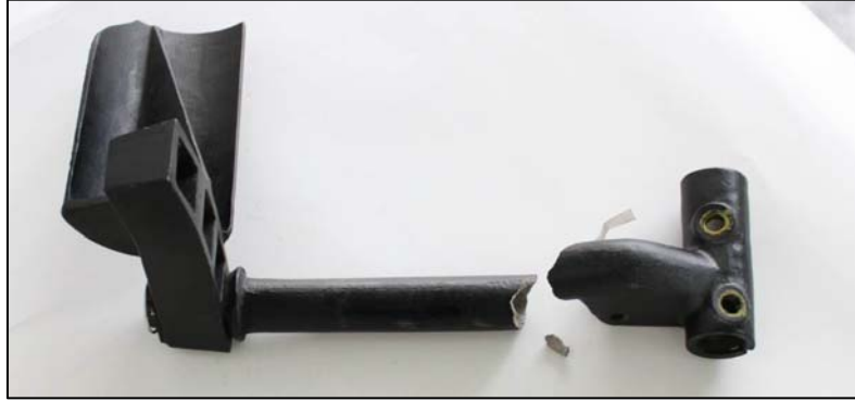
Fig. 4 Disassembled broken web of left pedal
