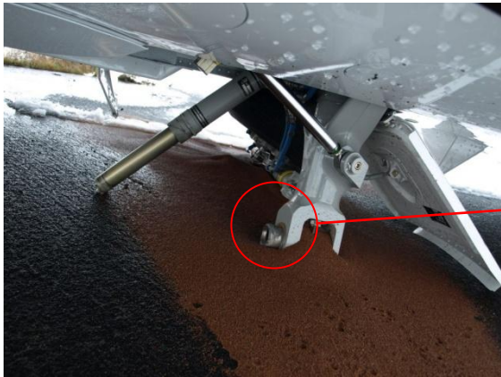
Fractured pin of left hand landing gear wheel axle
