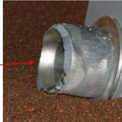
Fractured pin of left hand landing gear wheel axle
