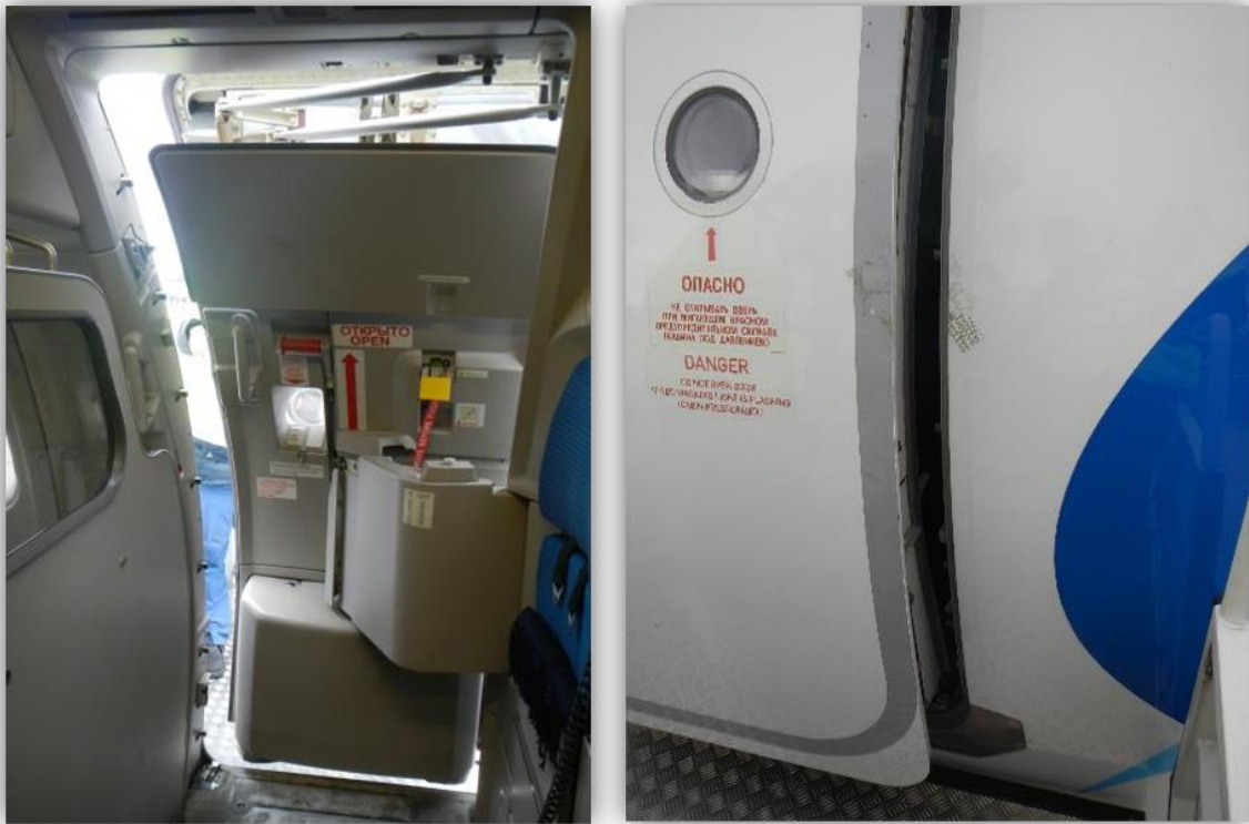
Fig. 2 The ajar front door from the cabin and from the vantage point of a person on the passenger stairs top platform
